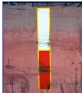
The "Pilot Mark": The line between the white and red sections marks 9 meters freeboard—the maximum continuous climb a pilot is required to make under SOLAS regulations.
